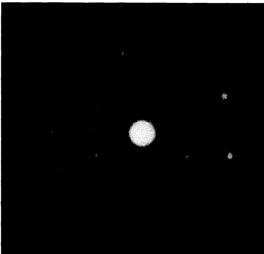
FIG. 4. Diffraction pattern of a catalyst region containing a large number of Pt particles.
