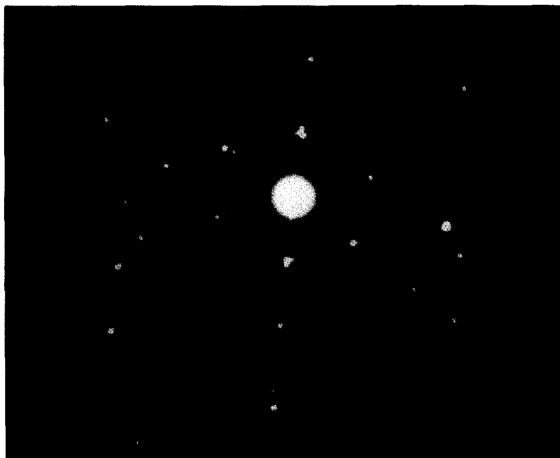
FIG. 6. Microdiffraction pattern of a H_2 -type single particle.
