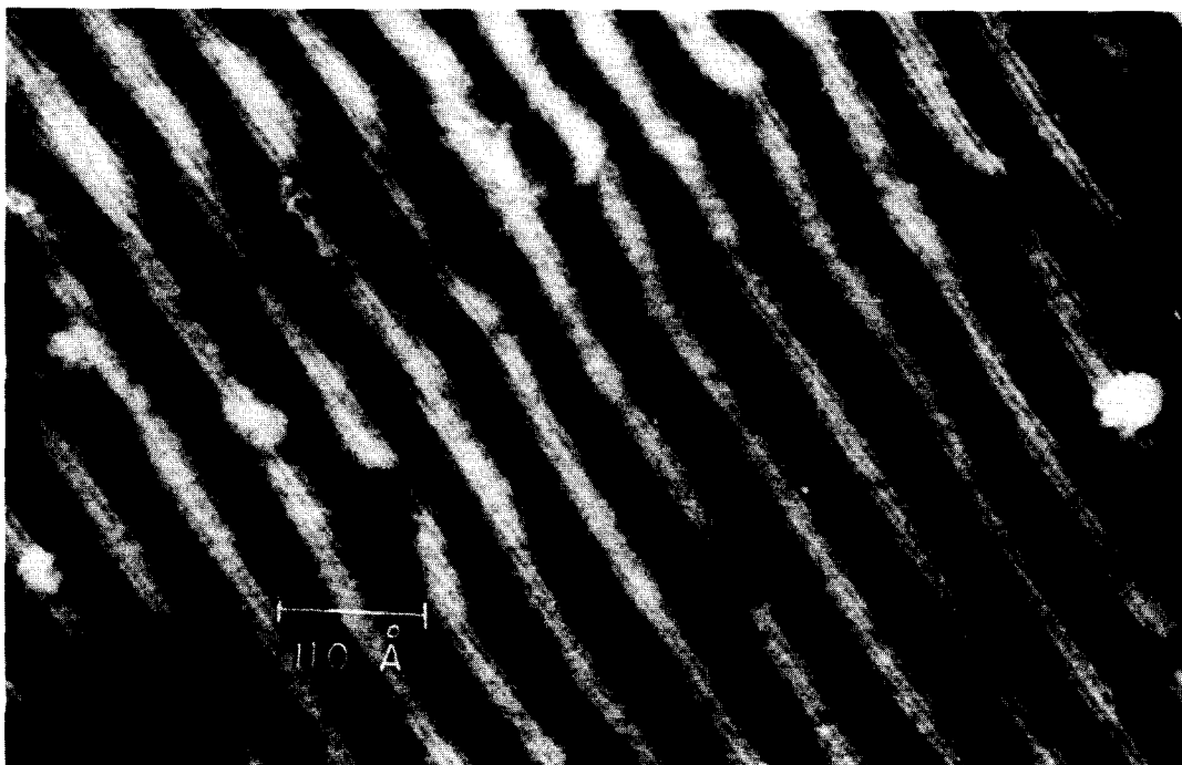
FIG. 2. Dark-field images of graphite showing a fine periodicity of 9.4 \text{ \AA} and a large one of \sim 72 \text{ \AA} .
